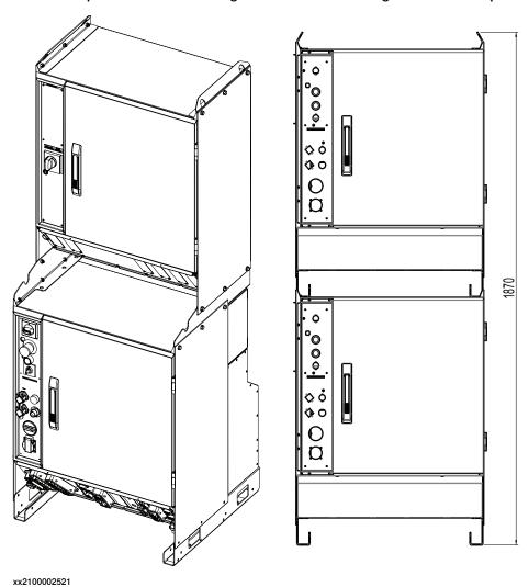
Height = 1870mm (Cabinet with lifting beam 970mm, cabinet without lifting beam 900mm)
